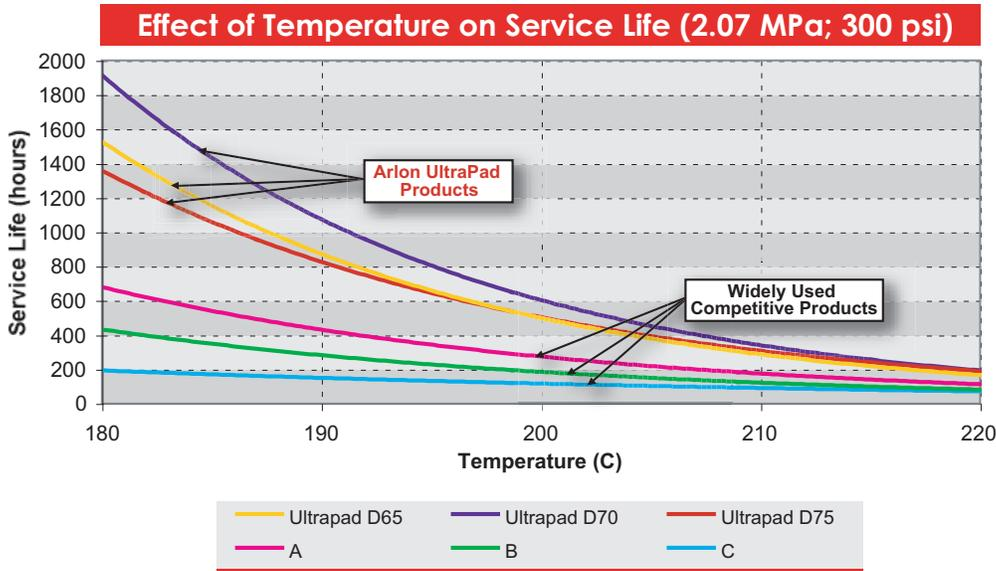
This chart provides press pad service life (one hour press cycles) over a temperature range of 180°C to 220°C. Three versions of UltraPad are compared to several competitive products, (A, B, C) when press cycled at 2.07 MPa.
